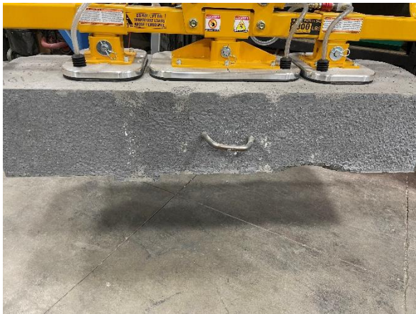
Figure 5 - One shear heel failed, one intact
