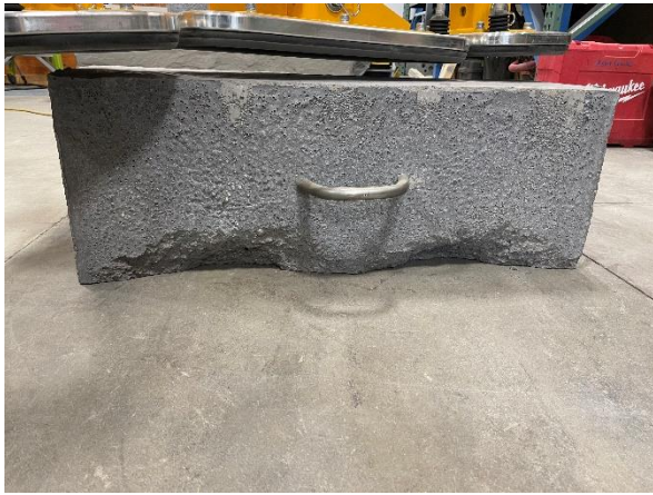
Figure 3 – Both Shear Heels sheared off bottom
