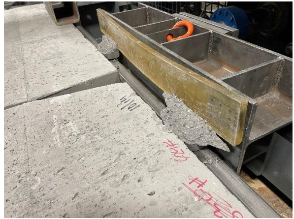
Figure 4 - Both shear heels left behind after test
