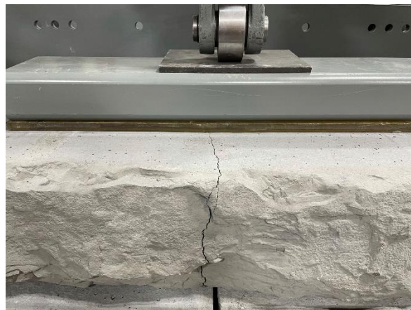
Figure 6 – Block cracked under high load
