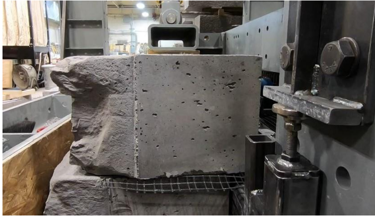
Figure 3 – Interface shear test setup
