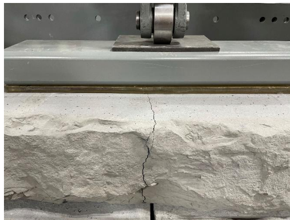
Figure 6 – Block cracked under high load
