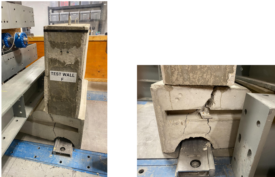
Figure 12 - Typical Failure Mode (taken from Test Wall F)
