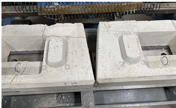
Figure 6 – Broken bottom blocks
