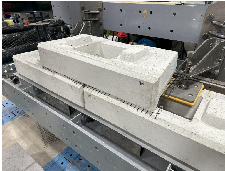
Figure 3 – Interface shear with geogrid inclusion test setup
