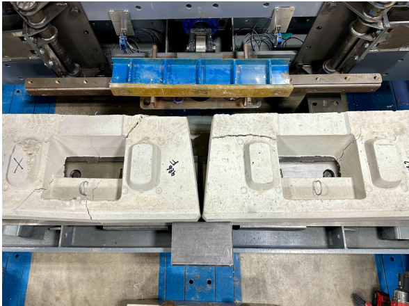
Figure 5 – Broken bottom blocks
