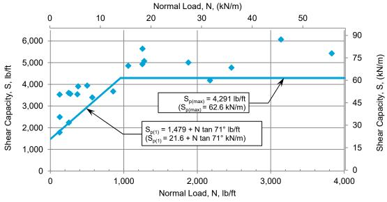
Peak Shear Envelope:  $S_p = 1,479 \text{ lb/ft} + N \tan 71^\circ \le 4,291 \text{ lb/ft}$  $S_p = 21.6 \text{ kN/m} + N \tan 71^\circ \le 62.6 \text{ kN/m}$
