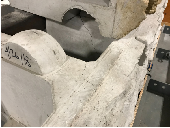
Figure 3 - Failure through block face
