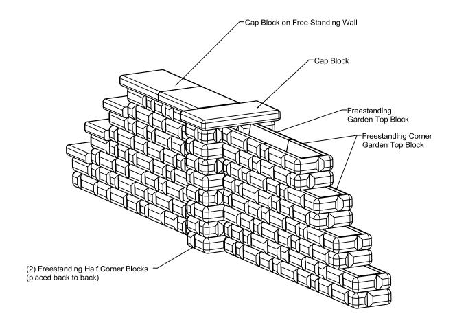
This sketch shows two options: On the near side of Pilaster, Freestanding Garden Blocks for vegetation, and solid cap blocks on the far side of the pilaster.
