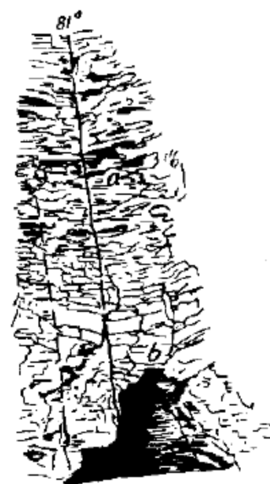
d. Slip plane parallel with dip extending from top of cave-in into top rock, showing breaking and slipping along plane
