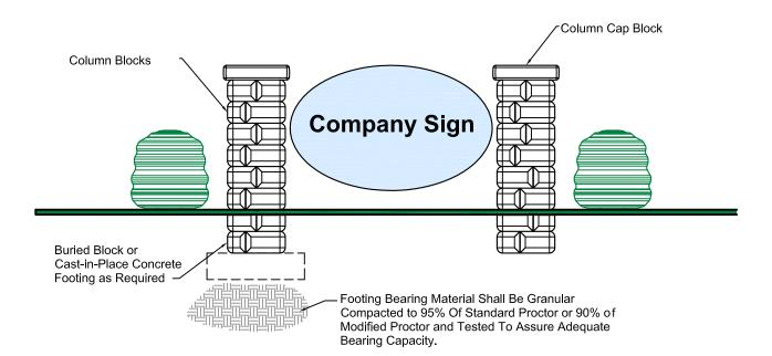
Steel reinforcement from footing and grouted column core as required by design (Typical for all columns) —
