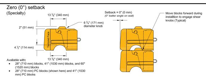
The block-to-block setback available with Redi-Rock is controlled by the size and location of the shear knobs (domes) cast into the blocks. While the 10" (254 mm) diameter knob and the 1 5/8" (41 mm) setback position is the most common configuration, Redi-Rock has three different knob sizes and three different locations available.
