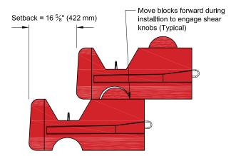
Redi-Rock has two options for large batter retaining walls. Both options are created by relocating the knob so that it is further back in the Redi-Rock blocks compared to our smaller batter walls (5° and less). There are two knob locations further back in the block which create the 9" (230 mm) setback block and the planter block. Blocks made with knobs in either of these locations almost exclusively use 10" (254 mm) diameter knobs.
