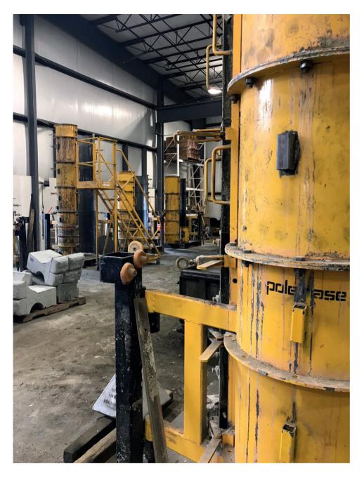
The days of cutting, welding, and grinding steel forms are over because Turner Concrete Product now uses Pole Base to create their custom, precast solutions for site lighting foundations. Having partnered with Toledo Edison back in the 1970s, Turner saw the benefits of the product but knew there needed to be a better way to manufacture them.
