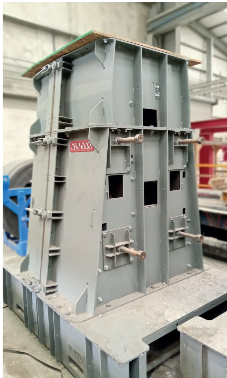
A Redi-Rock XL form set up to produce a 1320mm (52in) XL Hollow-Core Block. The form can also be modified to produce 1820mm (72in) and 2440mm (96in) blocks.
