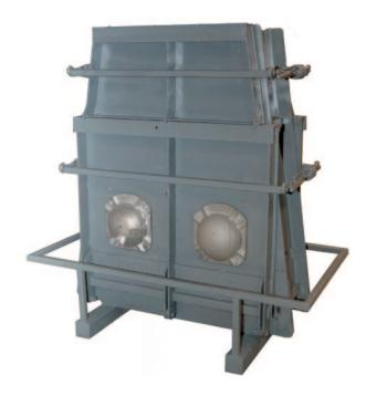
Many of the blocks manufactured for the Friday Harbour project were from the 60-inch series, where an extension is added to the standard Redi-Rock forming system.
