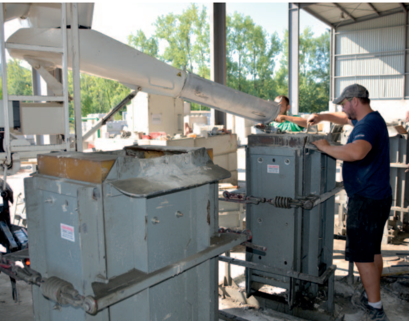
The BBlox team pours Redi-Rock freestanding forms to create freestanding wall blocks.
