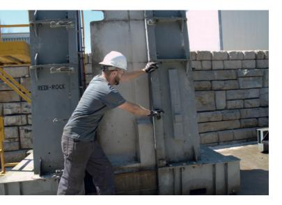
With the Redi-Rock forming system, no sophisticated equipment is necessary even for the largest of blocks. Forms can be poured using a Redi-Mix truck and demolded and inventoried using a forklift and hoists.
